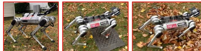
Fig. 7: Mini-Cheetah walks over different surfaces (grass, carpet, leaf surfaces) while carrying our sensor suite.
