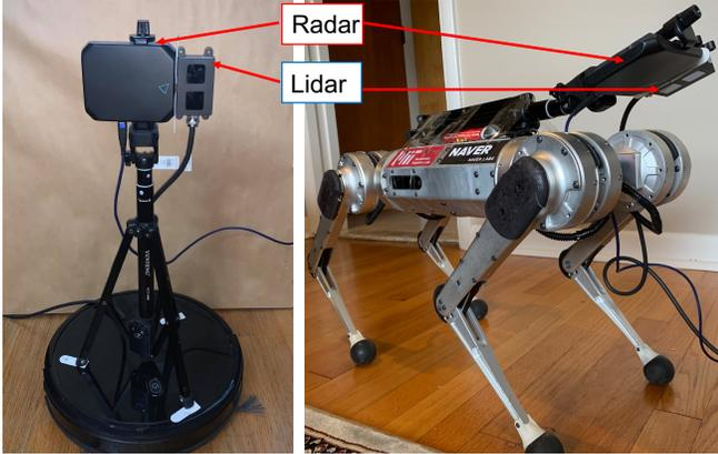
Fig. 1: Our Lidar-Radar sensor suite integrated with Vacuum Cleaning Robot and Mini-Cheetah quadruped robot [25]
